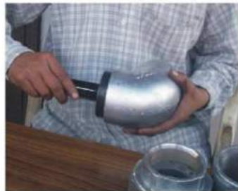
Fitting Inspection by use of standard thread gauge.
