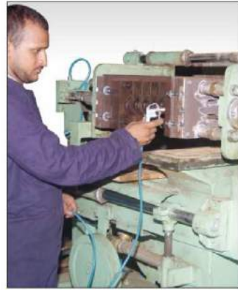
5. Moulds by Core Shooter Machine
